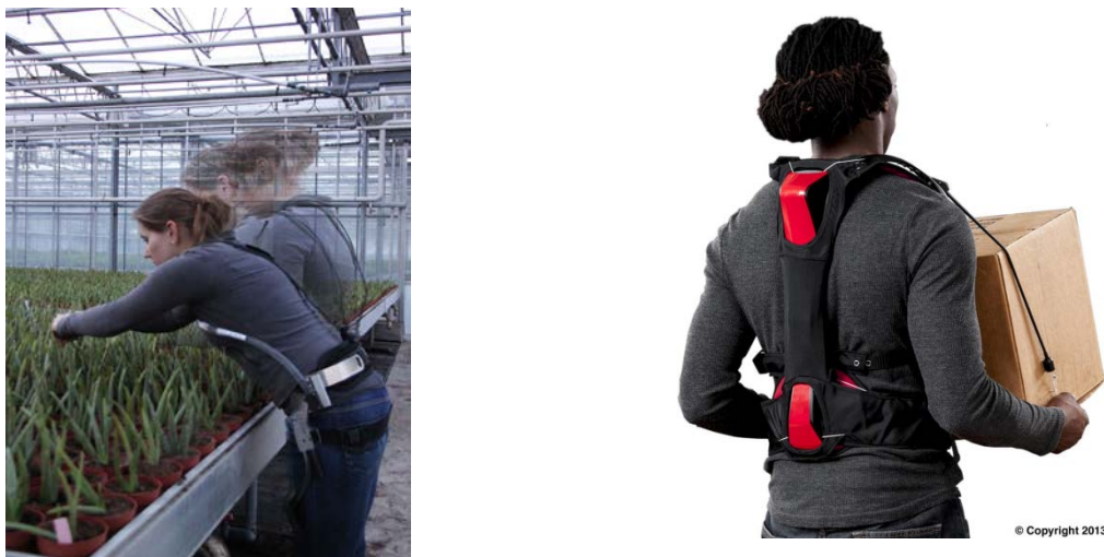
Figure 2: Devices assist the lower back when holding or carrying objects: (a) Laevo device uses springs at the waist to assist the body when leaning over, courtesy, Laevo, (b) Ergo-skeleton uses a clutch and cords to assist when lifting, courtesy, StrongArm.
